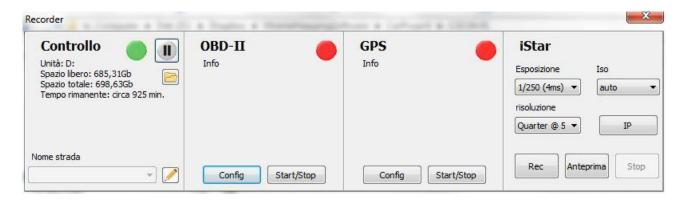
**GPS** receiver allows to georeference each of the panoramic images taken with the iStar, with a typical absolute accuracy of approximately 10 metres in ideal conditions. RTK upgrade, to increase the accuracy, is available on request.
